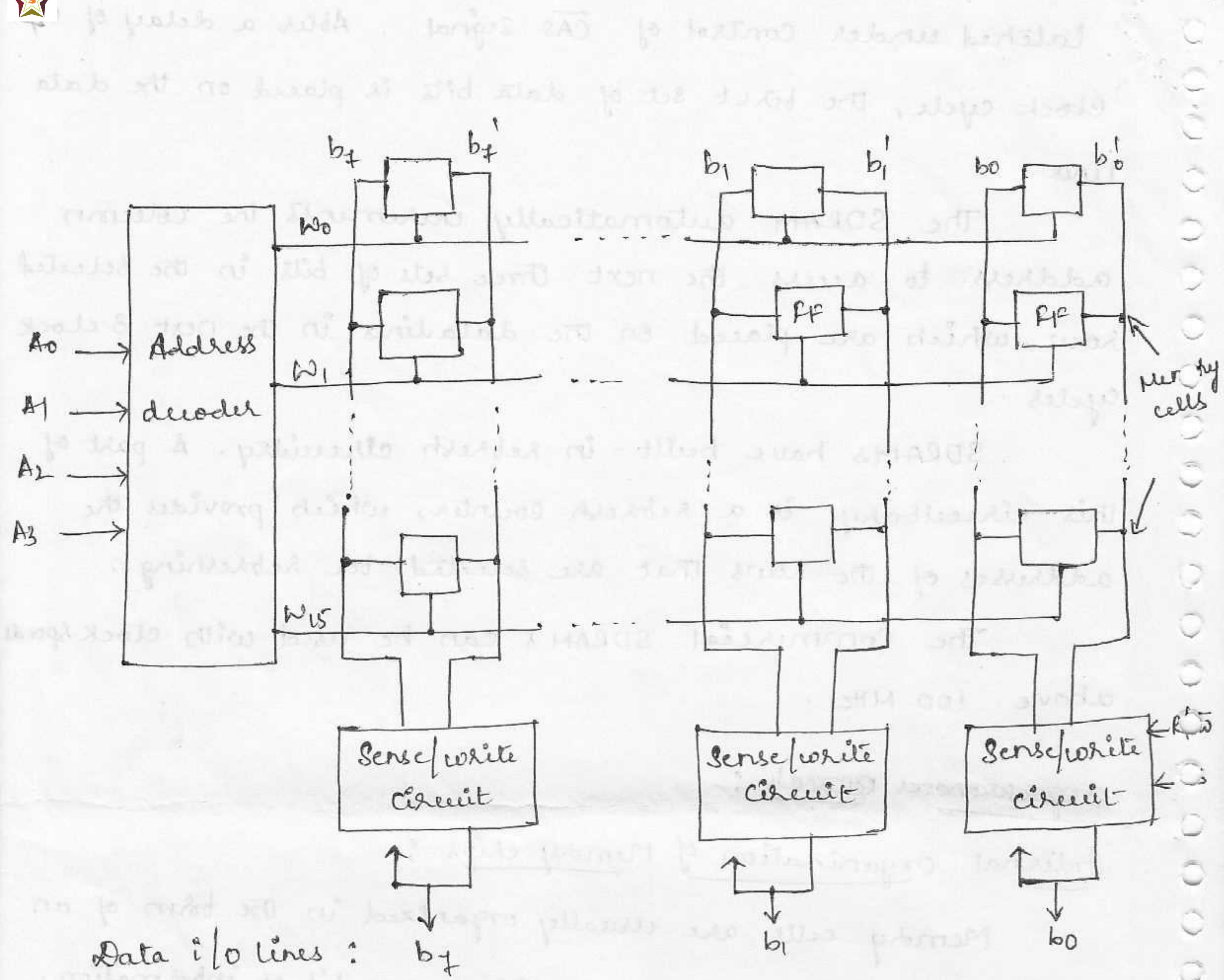
Word line and transmit this information to the o/p data bus. During a write operation, the sense/write circuit receive the information and store the cells of the selected record.
