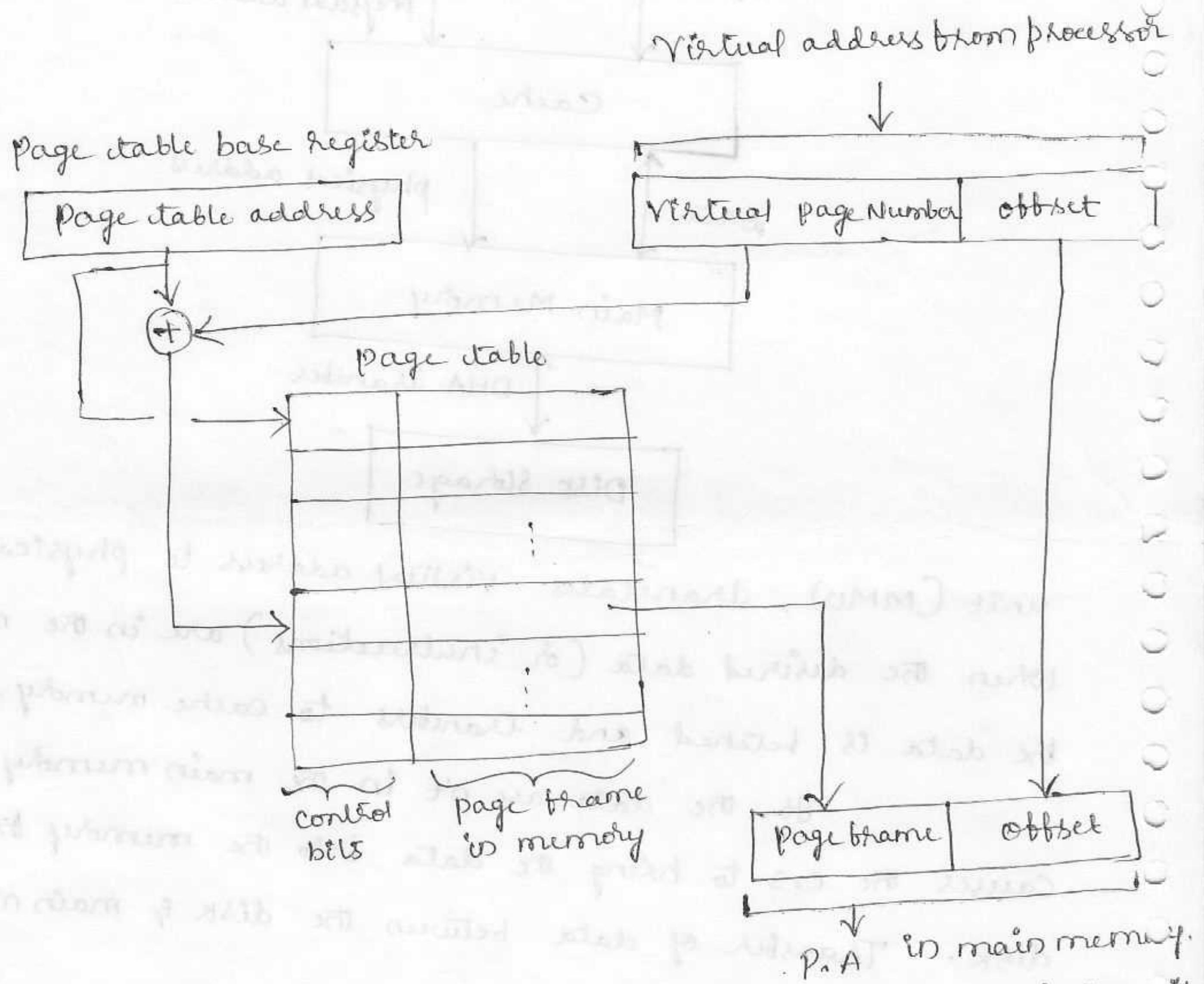
Each virtual address generated by the processor, whether it is for an instruction fetch or an operand fetch / store operation is interpreted as a virtual page number (High-order bits) followed by an offset (low-order bits) that specifies the location of a particular byte (or word) within a page. This interpretation creates an area in the main memory that can hold one page is called a 'page frame'. The starting <sup>address</sup> of the page table is kept in a 'page table base reg'.
