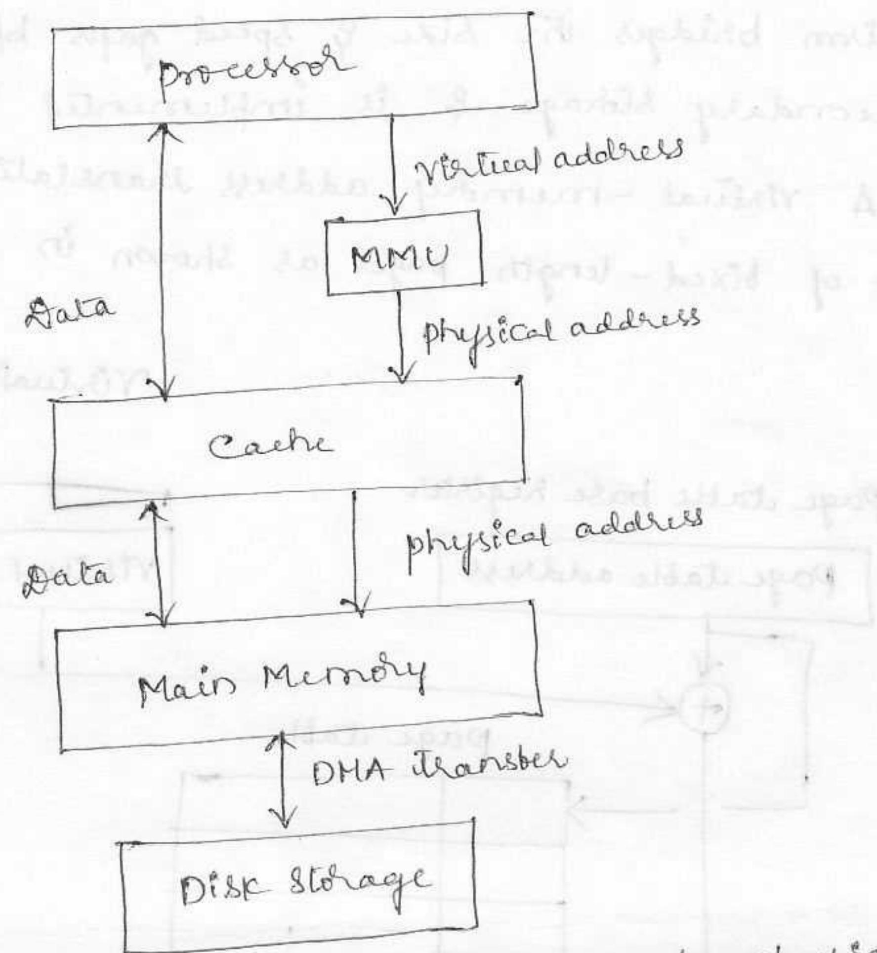
unit (MMU), translates virtual address to physical address. When the desired data (or instructions) are in the main memory, the data is fetched and transfers to cache memory. If the data are not in the main memory, the MMU causes the O.S to bring the data into the memory from the disk. Transfer of data between the disk & main memory is performed using DMA.
