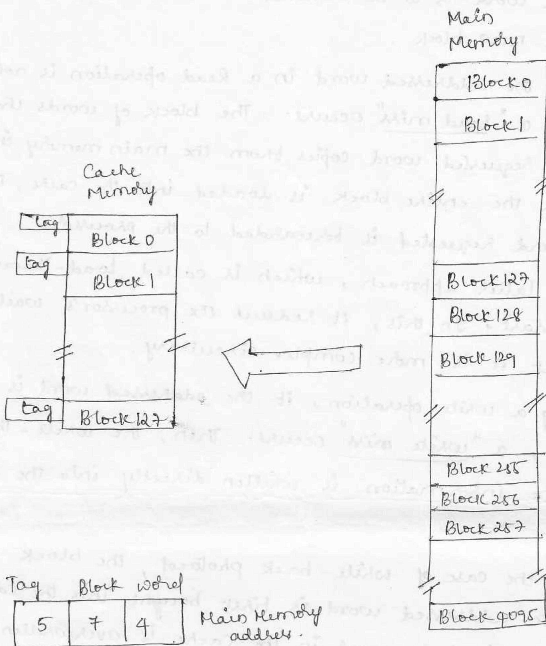
Since more than one memory block is mapped onto a given cache block position, contention may arise for that position even when the cache is not full.
