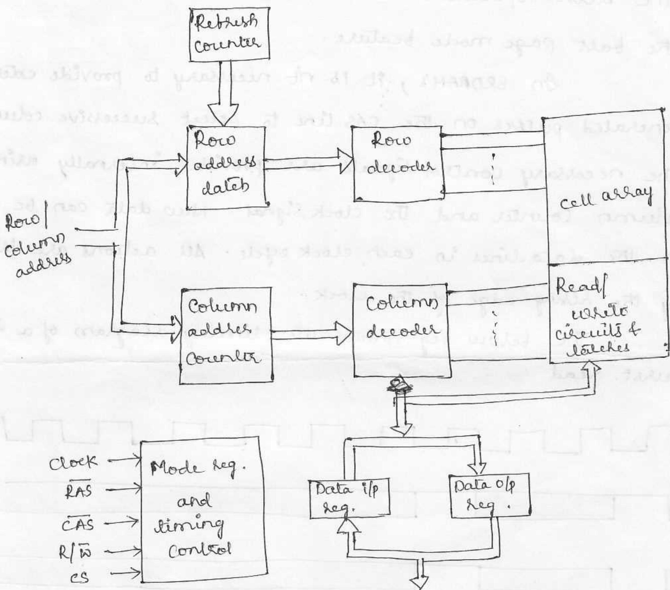
The address & data connections are buffered by means of registers. The O/p of each sense amplifier is connected to a latch. A read operation causes the contents of all cells in the selected row to be loaded into these latches. If an access is made for refreshing purposes but it will not change the contents of these latches and it will refresh the contents of the cells. Data held in the latches that correspond to the selected columns are transferred into the data o/p reg.
