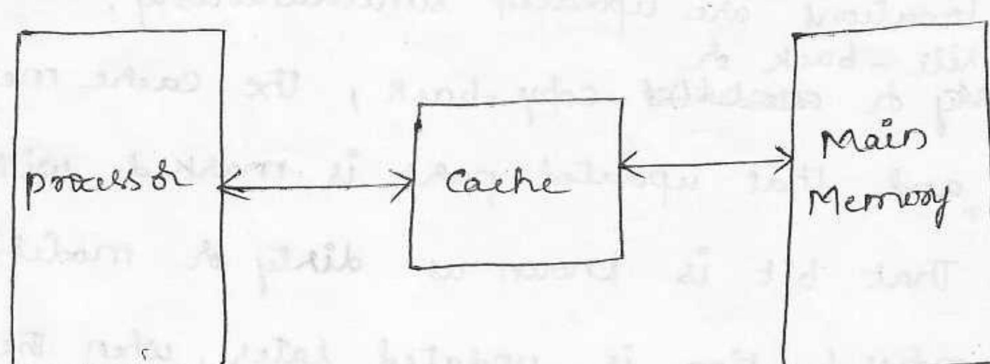
When a read request is received from the processor, the contents of a block of memory words containing the location specified are transferred into the cache one word at a time. When the program references any of the locations in this block, the desired contents are read directly from the cache. The cache memory can store a reasonable number of blocks at any given time, but this number is small compared to the total number of blocks in the main memory.
