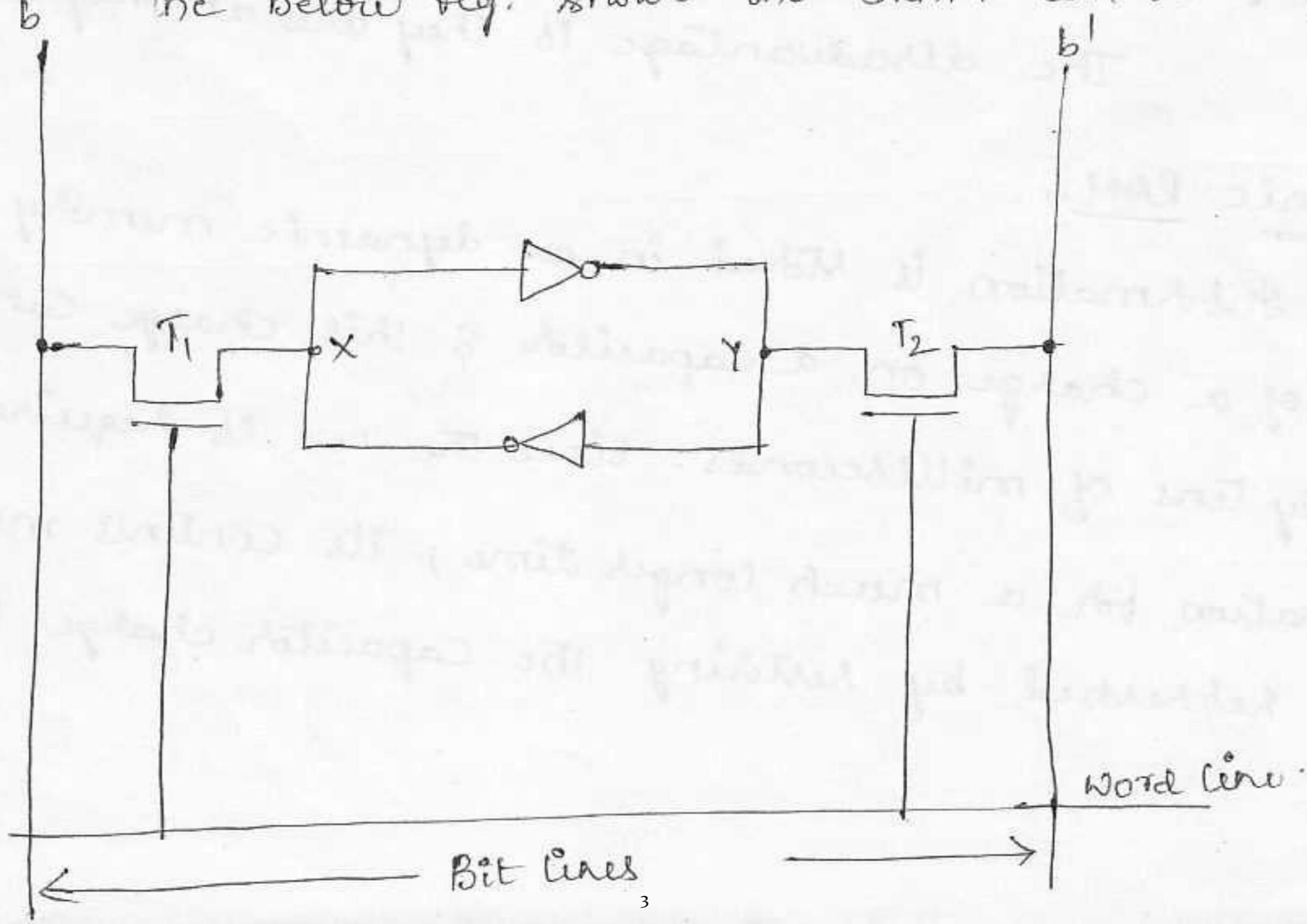
In the fig., the two inverters are cross-connected to form a latch. The latch is connected to two bitlines by transistors  $T_1$  &  $T_2$ . These transistors act as switches that can be opened or closed under the control of the word line. When the word line is at ground level, the transistors are turned off and the latch retains its state. For eg, let us assume that the cell is in state 1 if the logic value at point X is 1 and at point Y is 0.
