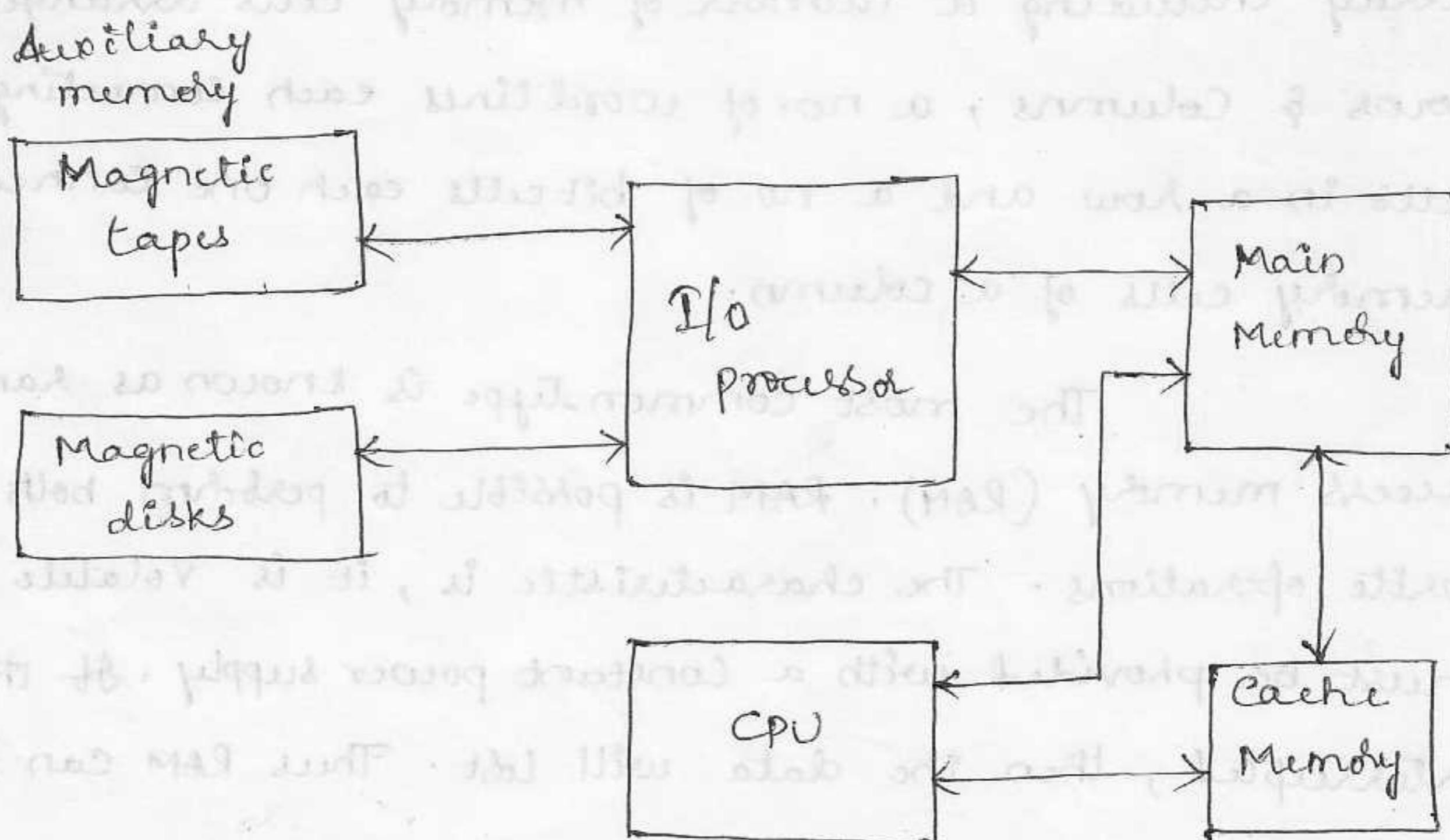
The Memory hierarchy system consists of all storage devices employed in a computer system from the slow but high-capacity auxiliary memory to a relatively faster main memory and
