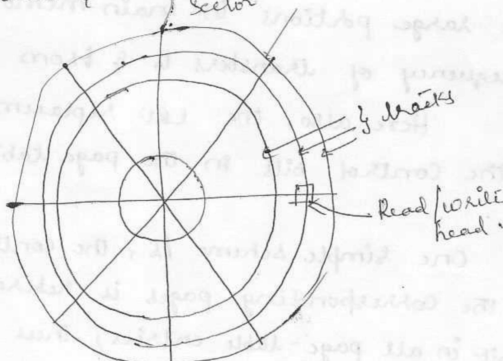
Some units uses a single read/write head for each disk surface. The track address bits are used by mechanical assembly to move the head into the specified track position before read/write. In other disk systems, separate read/write heads are provided for each track in each surface. The address bits can then select a particular track electronically thro' a decoder circuit.
