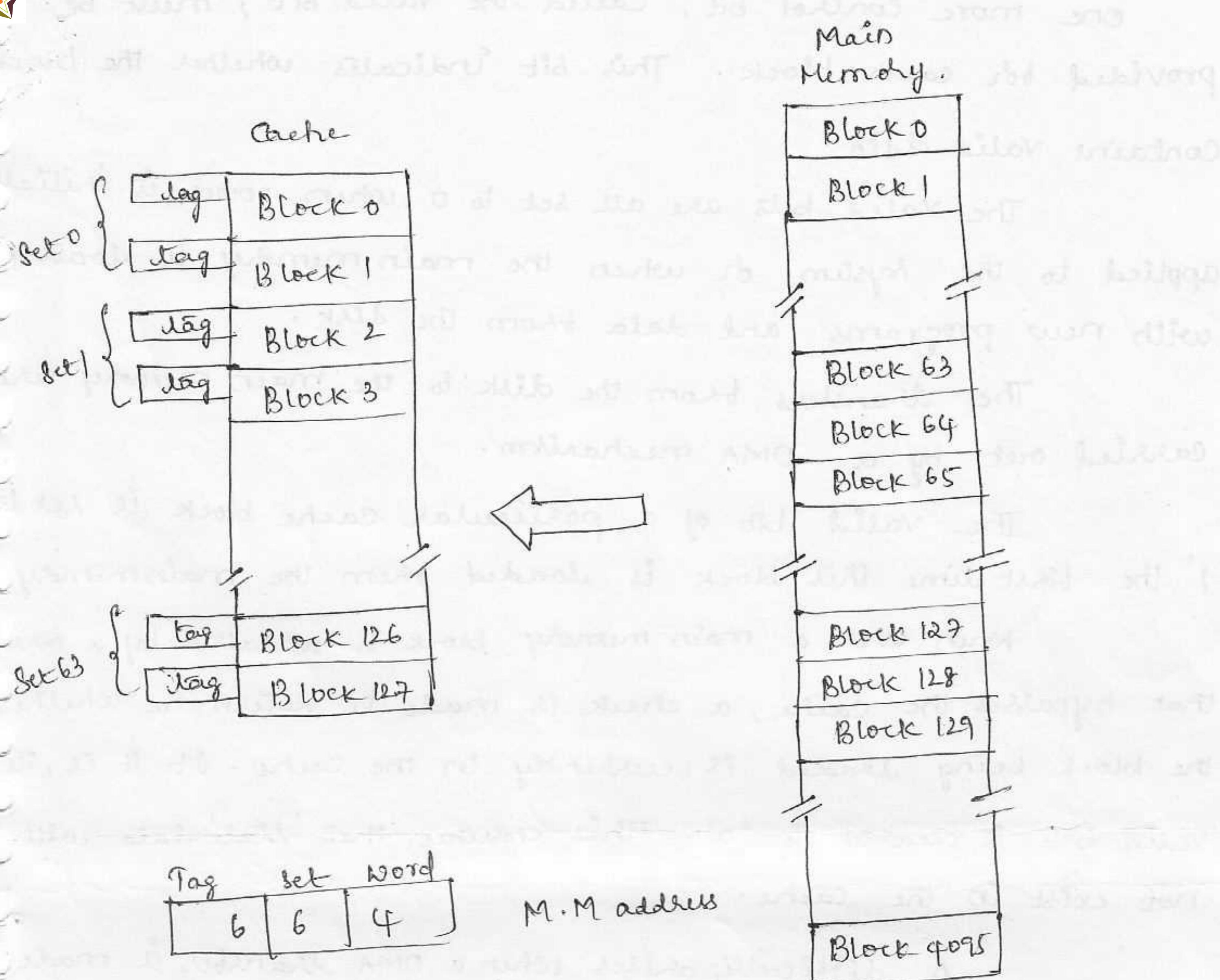
Having 64 sets means that the 6-bit set field of the address determines which set of the cache might contain the desired block. The tag field of the address must then be associatively compared to the tags of the 1120 block of the set to check if the desired block is present.
