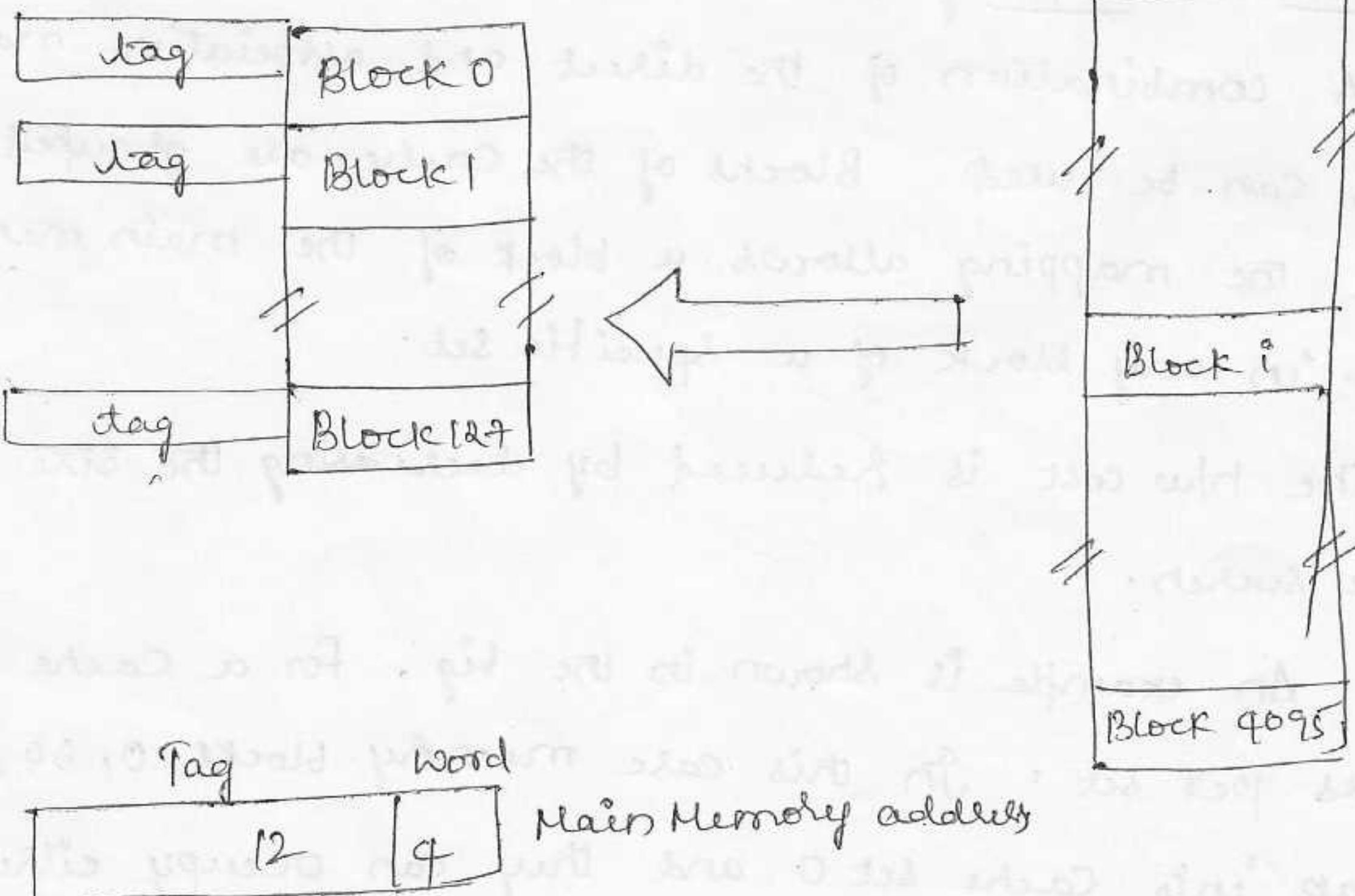
This is a much more flexible mapping method, in which a main memory block can be placed into any cache block position.
