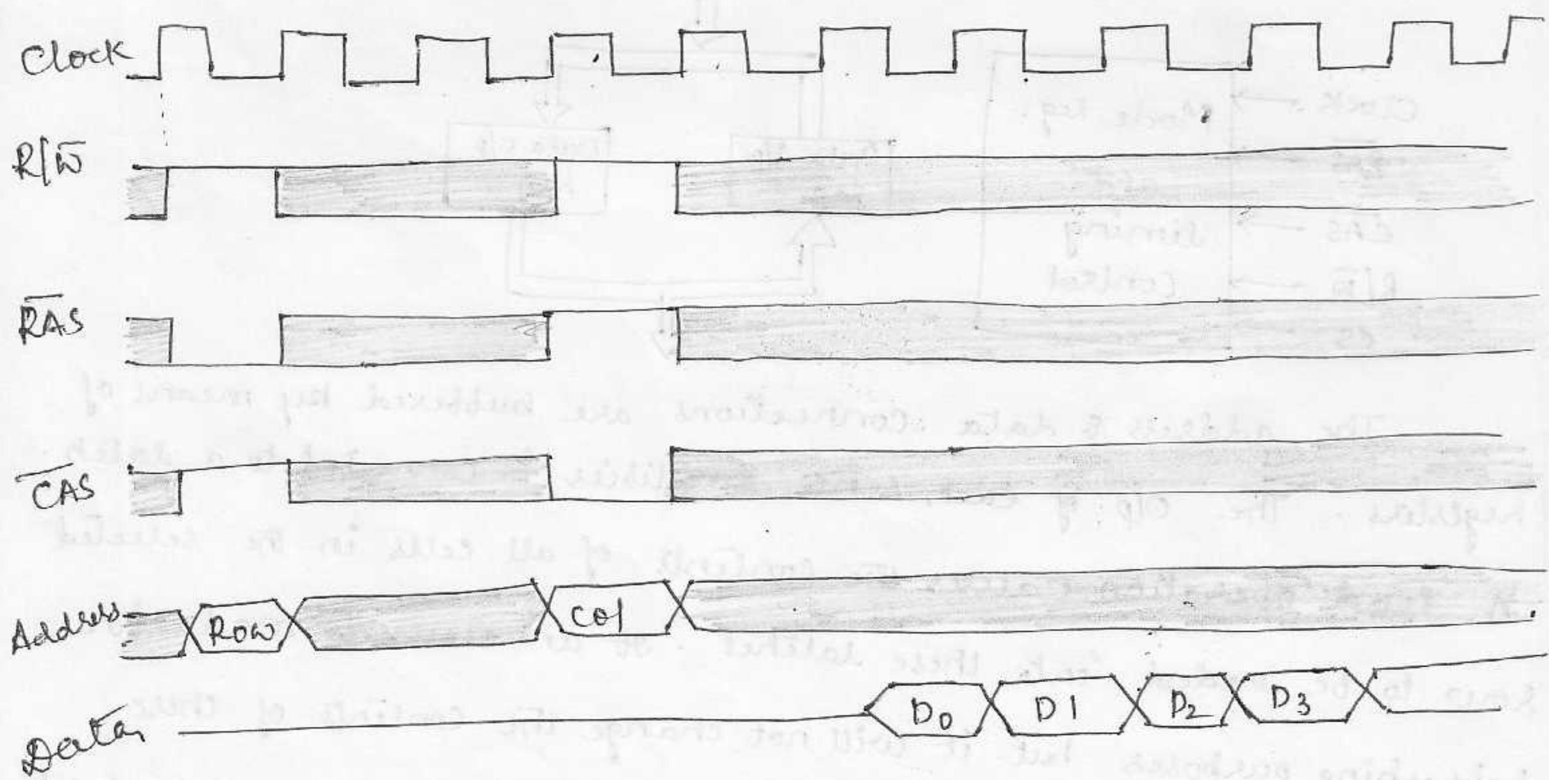
First, the row address is latched under control of the RAS signal. The memory typically takes 2 or 3 clock cycles to activate the selected row. Then, the column address is
