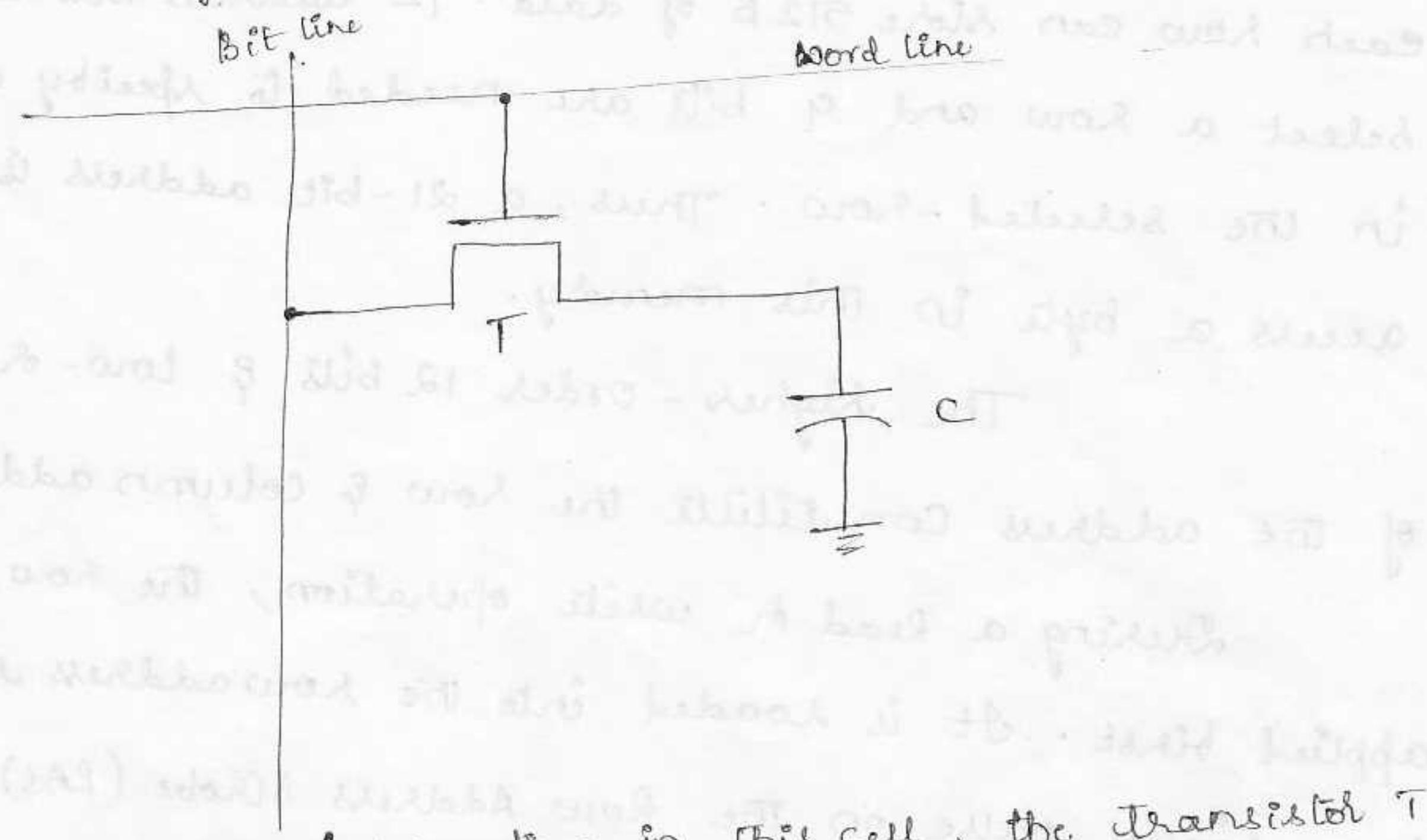
In order to store information in this cell, the transistor T is turned on and an appropriate voltage is applied to the bit line. This causes a known amount of charge to be stored in the capacitor. After the transistor is turned off, the capacitor begins to discharge.
